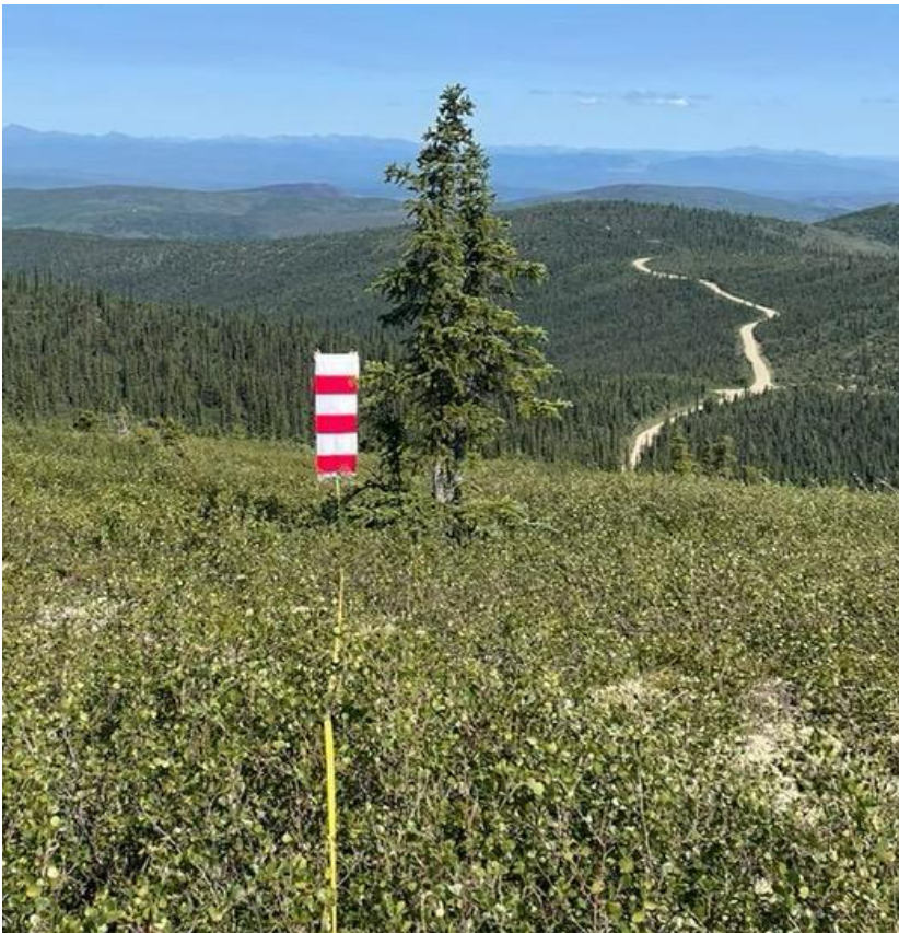
Figure 2. Photograph of a cover sheet survey from the plot center, demonstrating the point of view of the observer. The cover sheet is divided into alternating red and white rectangles (25 cm x 50 cm). The observer records percent of each rectangle obstructed by vegetation.
