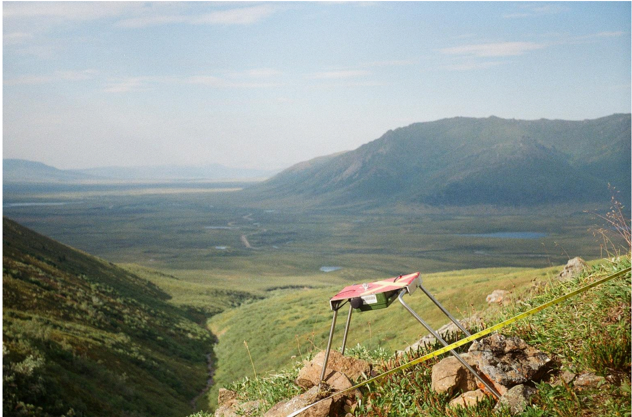
Figure 4. An ARU elevated off the ground by a metal stand at Mt. Boyle, Ddhäl Ch'èl Cha Nän. Photo by Charlotte Mittelstaedt.
