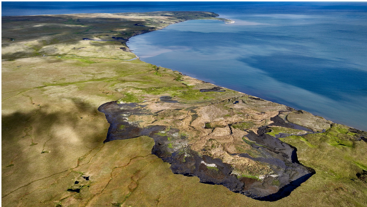
Figure 4. Drone surveys are allowing us to capture permafrost thaw, coastal erosion and vegetation change in high resolution on the island. This is an image of the biggest retrogressive thaw slump on the island in 2023.
