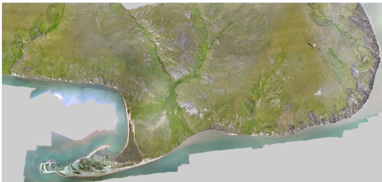
Figure 9. Drone imagery has been collected over the past three years on Qikiqtaruk to quantify vegetation across the landscape, to monitor disturbances such as permafrost thaw slumps and coastal erosion and to estimate above-ground carbon storage.
